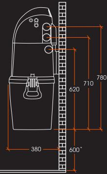
\* Minimum space recommended to allow the dust container to be emptied comfortably.
